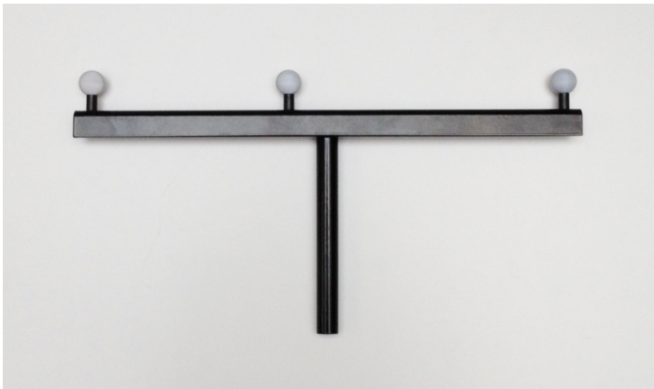
Figure 7.15: Registration device used for setting up multiple PST units
